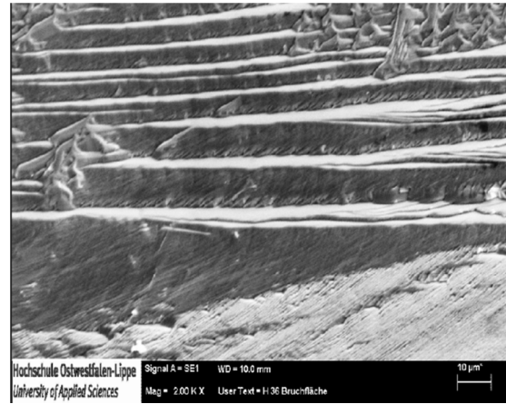
Fig. 3. The structure of CdSb(Te) crystals.
