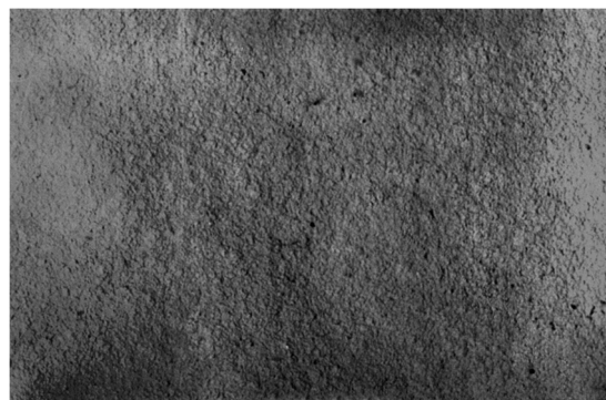
Fig. 9. Surface of Fe_{70,3}Ni_{29,7} alloy obtained with the pulsed current ( f = 30 Hz, Q = 32 ).
