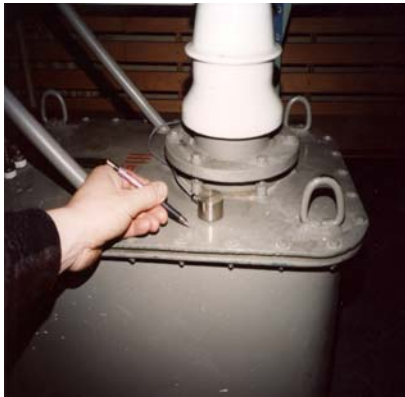
Fig. 2. Overall view of the transducer calibrated by the Hsu-Nielsen method, installed on a transformer.
