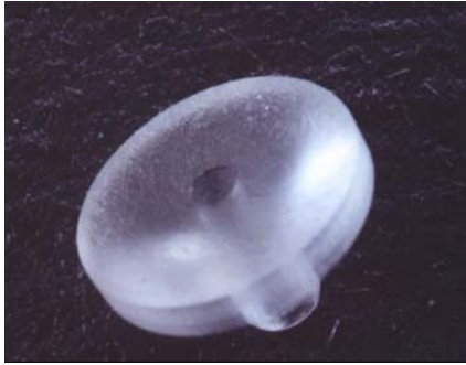
Fig. 1. Hsu-Nielsen calibration head.
