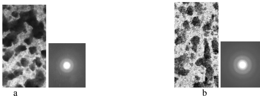
Figure 1. Film C 60 + WO 3 and microdiffraction from it (simultaneous deposition): a – initial sample, b – after annealing at 573K.
