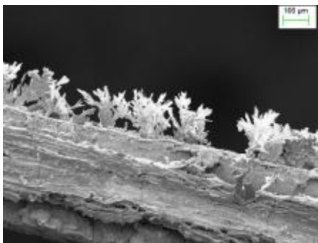
Figure 1. Bush-like oxide structures on the surface of tungsten filament.
