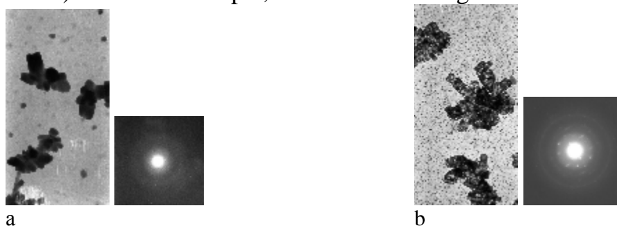
Figure 2. Film C 60 + Cu and microdiffraction from it (simultaneous deposition): a – initial sample, b – after annealing at 573K.
