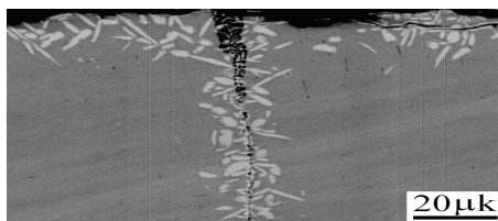
Fig. 2. SEM image of cross-section FeCoCrNiVAl alloy after annealing at 1273 K /2h
